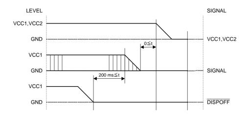
Please maintain the above sequence when turning on and off the power supply of the module. If  $\overline{\text{DISPOFF}}$  is supplied to the module while internal alternate signal for LCD driving (M) is unstable, DC component will be supplied to the LCD panel. This may cause damage the LCD module.
